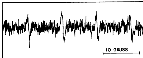
Figure 3. ESR signal following UV irradiation of bleached K-ethylamine solution; Strand Labs Model 601 X-band spectrometer, 3200 gauss; room temperature.
